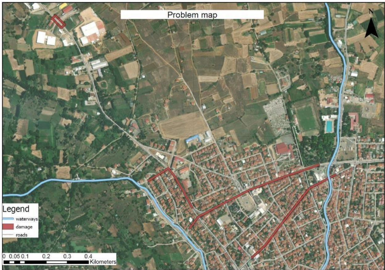
17. Figure: Damaged drainage system elements
